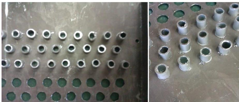
When I fitted all the tubes I glued them to the metal cover. The next step was making a big hole for the “rotor wheel” cover. For this I drew the dimensions and used a hammer and chisel to make the hole. I drilled a hole on each corner for bolts.
