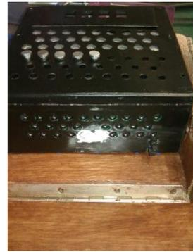
After this the cover was spray painted black. The inside was also painted so the metal dust which collected inside there was captured and could not damage the PCB.
